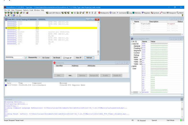
The next step is to run the ITH macros that enable the Trace Hub and hide it from the OS. Fortunately, SourcePoint comes equipped with a macro button built in to make this process easier, At the top of the screen, you'll see a button labeled NPK and EnableTraceHub. Click on it. Wait about five seconds.
