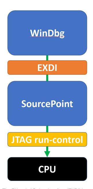
The EXtended Debug Interface (EXDI) is used to connect a WinDbg debugging session to an existing SourcePoint JTAG-based connection to a target.
