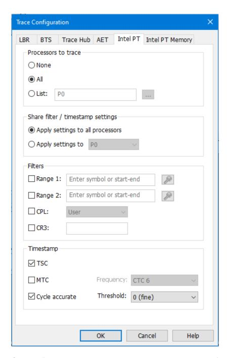
Click on "All" Processors to Trace", or select a processor from the list. Ensure both  ${ t TSC}$  and  ${ t Cycle}$  accurate are enabled.
