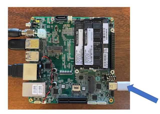
For the v0001 board, the Type-A/A cable can be plugged into any of the three USB3.0 ports (the blue jacks) available. All three jacks support DCI. The USB2.0 port (the black one) does not support DCI.
