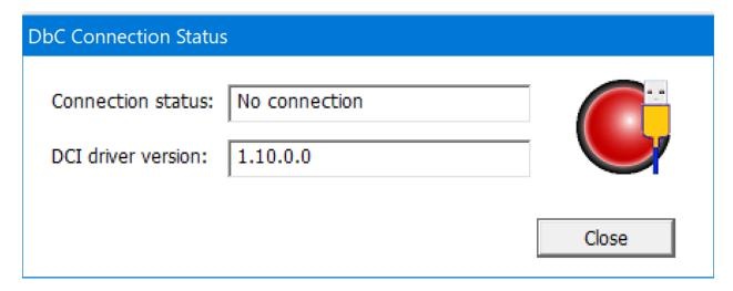
For the v0000 board, ensure that the Type-C cable is firmly connected to both the host and target, power up the UP Xtreme i11. In a moment the ball should turn green:
