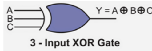
Figure 5: 3-input XOR gate
