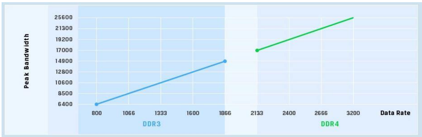
Figure 1: DDR4 peak bandwidth vs. data rate
