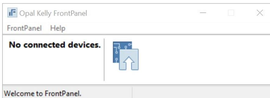
Plug in the USB cable to the Opal Kelly Board and to the host where the FrontPanel and ScanWorks resides. The FrontPanel will look similar to the interface shown below.
