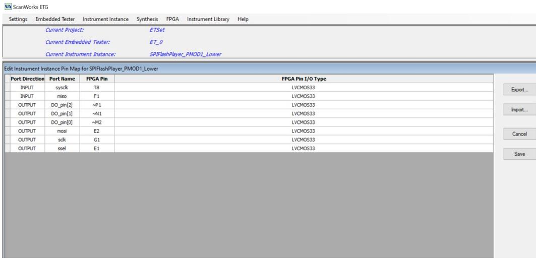
The three DO\_pins declared above are static pins with a default state of 1 due to the ~. Since they are declared in this instrument, these pins can be set high or low within the ScanWorks SPI IP action, just as they could be in a standard SPI action. In the Opal Kelly design these pins are connected to D6, D7 and D8. Removing the ~ will illuminate these LEDs when the SVF is loaded into the FPGA.
