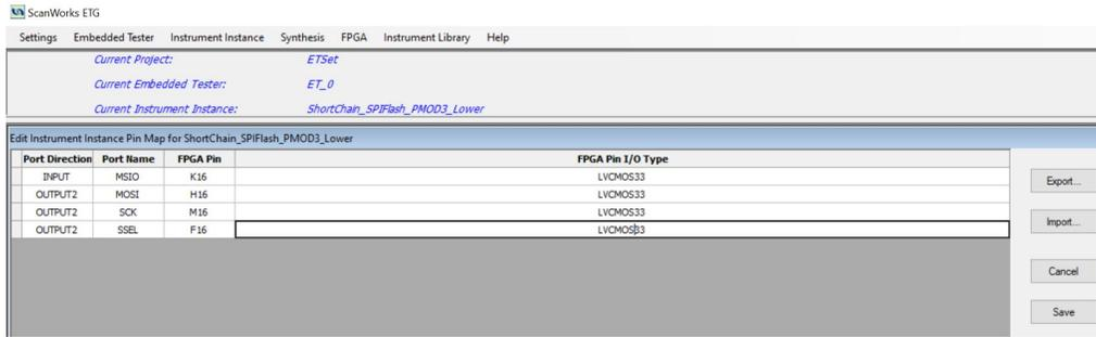
II. Add an SPI FlashPlayer instrument to program the SPI flash device at PMOD1, lower position.
