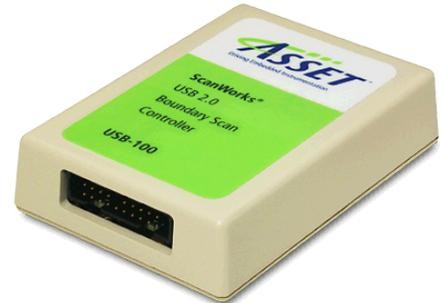
The compact USB-100 is about the size of a deck of playing cards. Standard, off-the-shelf USB 2.0 mini-B cable connects the USB-100 to a PC, making it easy to transport and connect. A large pod is not needed to connect ScanWorks to a UUT in the field or in manufacturing environments.
