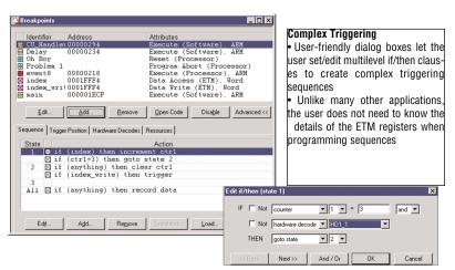
Deep/fast trace. With the Arium LX-1000 for ARM trace port analyzer, SourcePoint for ARM delivers trace depth up to 8 GBvtes with a capture rate up to 680 MHz.
