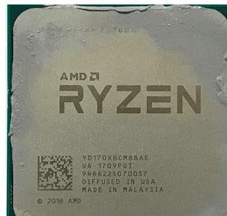
The “UA 1709PGT” on the second line designated that this was a work week 09 production run, and all CPUs prior to WW25 are expected to have the segfault issue.
