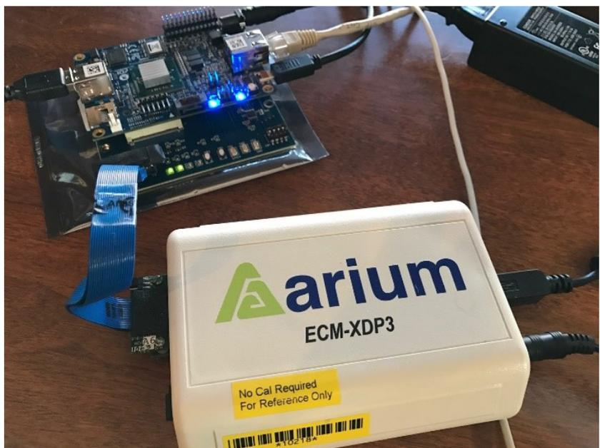
The emulator plugs into the standard 60-pin XDP header on the Debugger Lure, which in turn plugs into the HSE header on the bottom of the MinnowBoard. It was very easy to set up.
