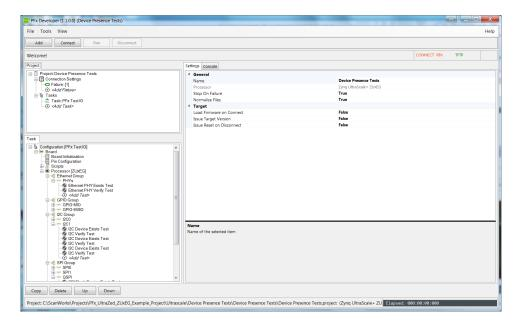
16. This action checks for the presence of the Ethernet PHY, The flash device on the QSPI port, I2C devices and the presence of the MMC device. Click on the Connect button, then the Run button.
