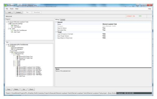
20. This action tests for the presence of the Ethernet PHY, does loopback tests on the ethernet MAC and loopback tests on the Ethernet PHY. Click on Connect and then on Run.
