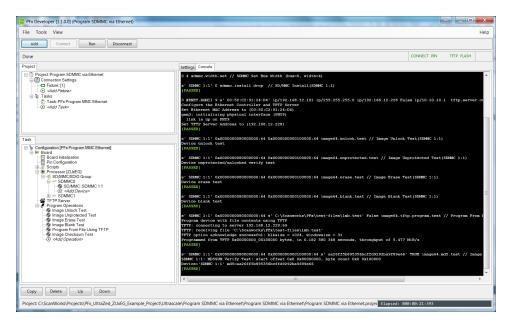
30. Note that in the example above, the SD/MMC card was programmed at a rate of 5.47 MiB/second. Close the Developer interface, and click on the Run button to the left of MMC Programming using Ethernet.
