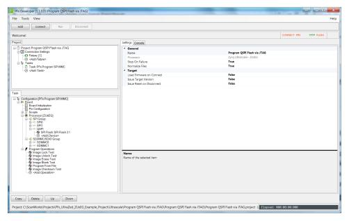
32. This action tests for the presence of a flash memory device on the QSPI port, Erases the flash, does a blank check on the flash, Programs the flash with a test file over JTAG, and then tests the checksum of the range of flash memory that was programmed.
