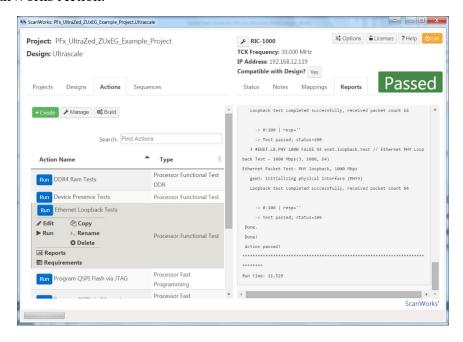
22. Right click on QSPI Programming via Ethernet to open Developer interface for the QSPI using Ethernet action. This action tests for the presence of a flash memory device on the QSPI port, Erases the flash, does a blank check on the flash, Programs the flash with a test file over Ethernet, and then tests the checksum of the range of flash memory that was programmed.
