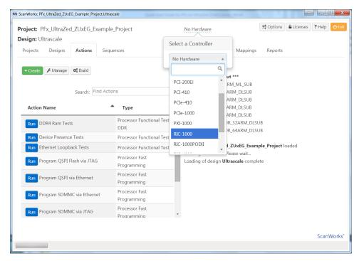
8. Configure the RIC-1000's ip address, and select a TCK Frequency of 30 MHz. Note that flash programming performance over JTAG is directly affected by the TCK frequency. The higher the TCK Frequency, the better the programming performance. Click OK.
