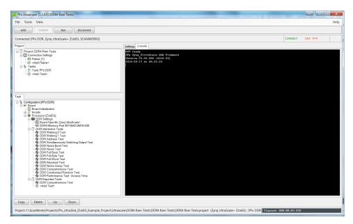
12. You can manually run any of the tests in the DDR Interactive Tests group by right clicking on it and selecting Run. Click on the Run Button near the top of the window to run the test(s) that are in the DDR Exported Tests group.
