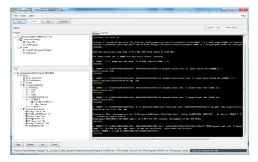
36. Note that in the example above, the SD/MMC card was programmed at a rate of 113.0 KiB/second. Close the Developer interface, and click on the Run button to the left of Program SDMMC Programming via JTAG. This concludes the Developer portion of this guide.
