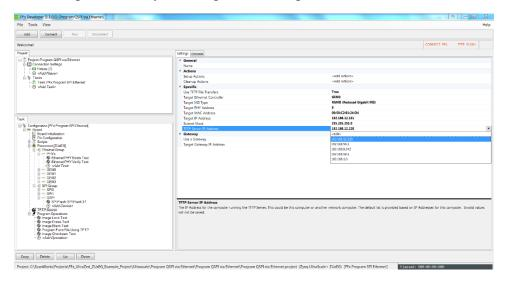
24. Now configure the ipaddress of the UUT by entering the desired value in the field to the right of Target IP Address. Configure the subnet mask. Save the project.
