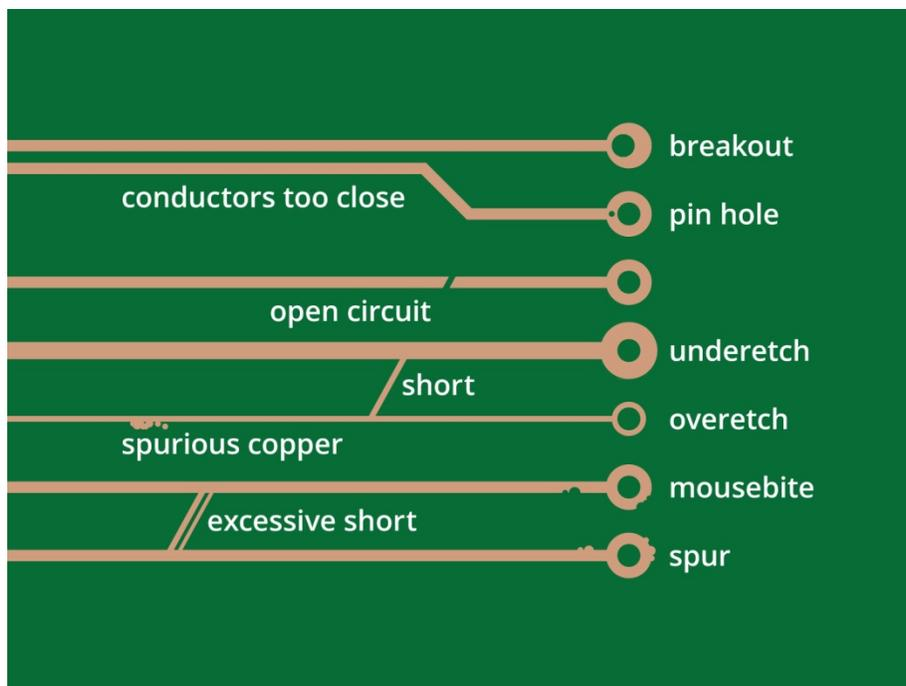
Figure 1: Manufacturing process variances can cause a number of defects.
