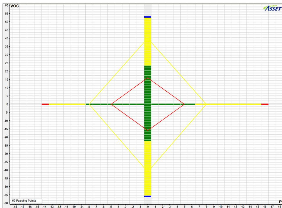
**Figure 3: This composite view of a cross margin test shows where all lanes are passing (green), some lanes are failing (yellow) and all lanes have failed (red). Blue indicates some lanes were still passing at the maximum allowed range.**
