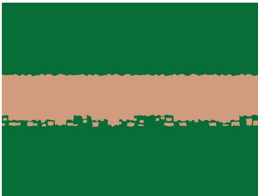
**Figure 2: This illustration of a trace on an inner layer of a PCB shows the roughness of the copper on the upper and lower surfaces of the trace.**
