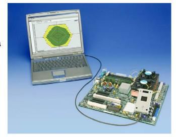
NBT test technologies make use of the JTAG port (that is, the IEEE 1149.1 Boundary Scan Standard's Test Access Port) to access the circuit board, but other interface technologies can serve in the same role. In addition, NBT involves embedded test intellectual property (IP) in chips and on circuit boards. With boundary scan, for example, chips that are compliant with the standard include a few test registers, and circuit boards are architected to enable boundary scan access and test.
