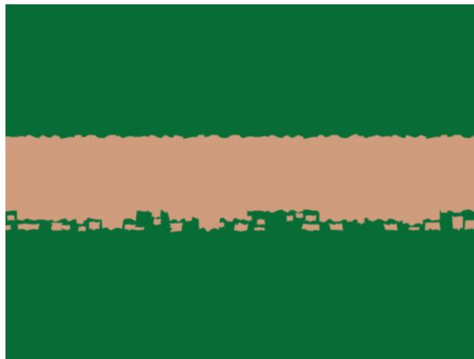
**Figure 8: Stripline cross-section, illustrating trace surface roughness**
