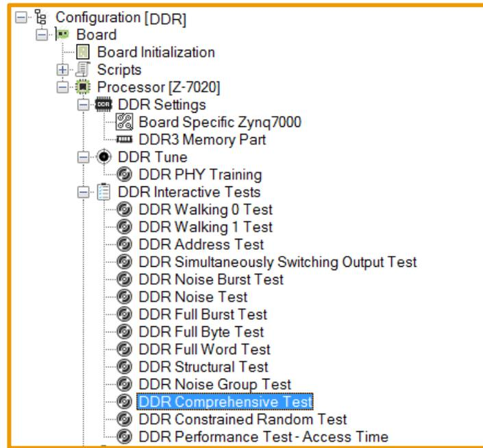
Figure 20: DDR Memory Test Prior to Tuning
