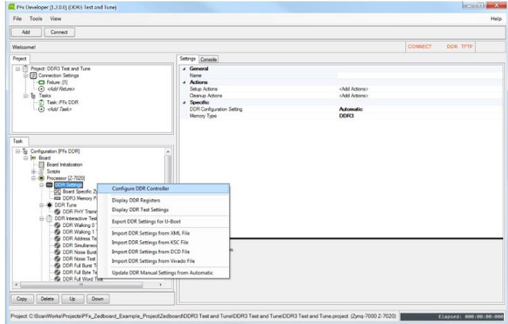
Figure 4 Configure DDR Controller and device initialization
